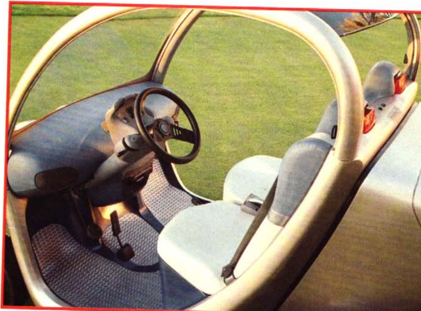
Sturges's car's tipped ovoid form, generated by the ellipse that will circumscribe a seated human, allows splendid visibility and easy ingress and egress. The instrument panel (above right) is simply functional.
